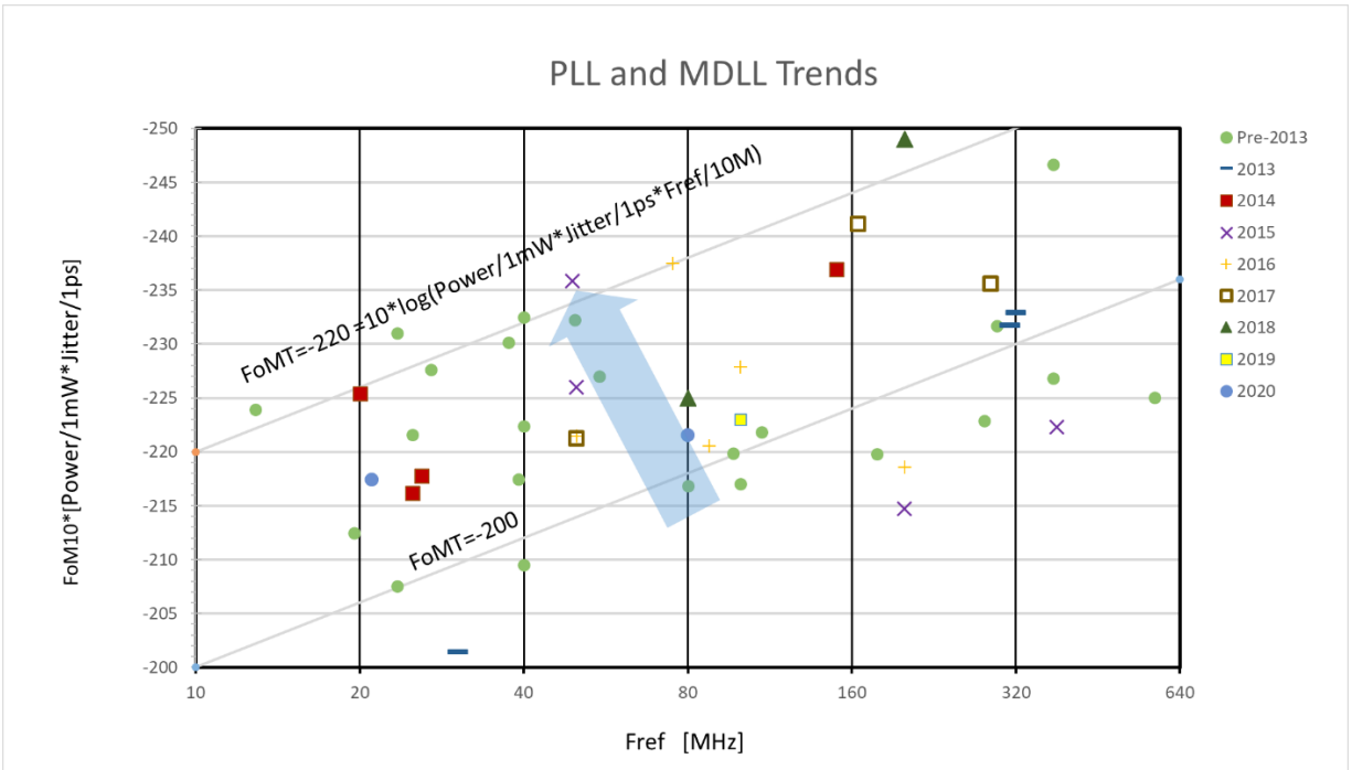
Figure 24. PLL and Multiplying-Delay-Locked Loop (MDLL) trends.
